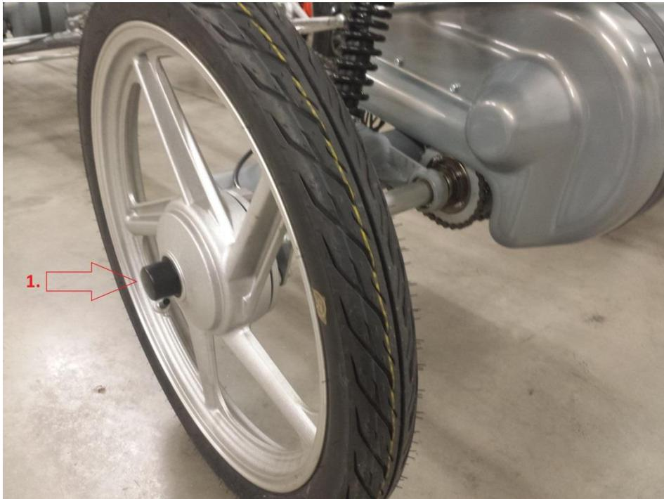
Figuur b: Axle with freewheel sprocket
